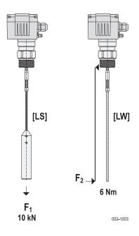
Wire rope probe [LS] maximum tractive force  $F_1 = 10 \text{ kN}$ Rod probe [LW] maximum side load  $F_2 \times LW = 6 \text{ Nm}$
