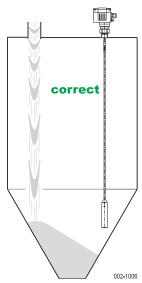
Choose the mounting position in that way the probe will not be hit by the filling flow rate.
