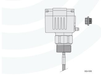
Condensate protection valve for insertion into a threaded hole. A watertight but vapour-permeable membrane prevents condensate formation in the interior of the housing.
