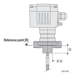
Level indicator with conical adapter and corresponding groove nut for dairy coupling.
