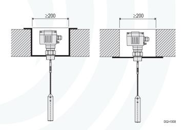
By mounting in a concrete floor the process connection should aligned with the bottom edge of the floor.
