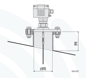
Protruding nozzle diameter **[G]** ≥100 mm
