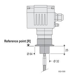
Level indicator with clamp connection. For installation of the level indicator into containers which must be cleaned for hygienic reasons, or for quick removal of the indicators when the vessels are changed.
